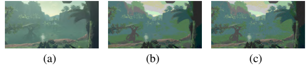
Figure 5: (a) Input image before preprocess; (b) Image after quantization; (c) Gaussian noise is added to (b).
